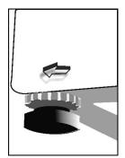
• Adjust the feet upward and downward by rotating them clockwise and anti clockwise.
